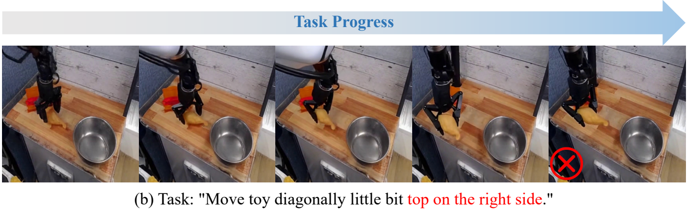
Fig. 3: Failure Cases of Large-Scale Video Generation Model (NVIDIA Cosmos-Predict2.5). Despite being trained on massive datasets, the model still exhibits significant issues in physical reasoning for robotic manipulation. (a) The model fails to follow the instruction “on top of”, placing the block next to the target instead. (b) The generated motion does not align with the “top right” directive. Crucially, in both cases, we observe morphological deformation of the robot arm (e.g., the gripper shape distorts over time), indicating a lack of rigid-body dynamics understanding. This suggests that simply scaling up visual generation does not automatically solve the need for explicit dynamics modeling (e.g., optical flow) in robotics. For visualizations of correct predictions generated by our proposed method, please refer to Figure 8 and Figure 9 in the main manuscript.
