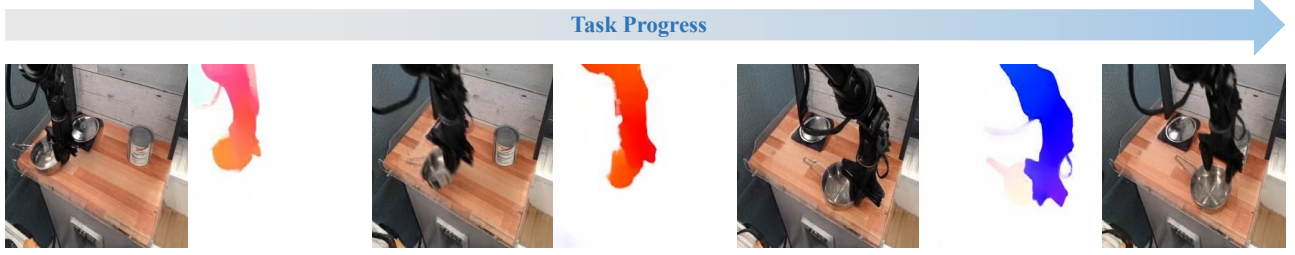
Fig. 2: Robustness on Textureless/Reflective Objects. We visualize the optical flow predictions while manipulating a stainless steel pot. Despite the object being textureless and metallic, RAFT accurately predicts dense flow across the entire object surface, demonstrating that the model effectively propagates motion cues from boundaries to textureless regions.
